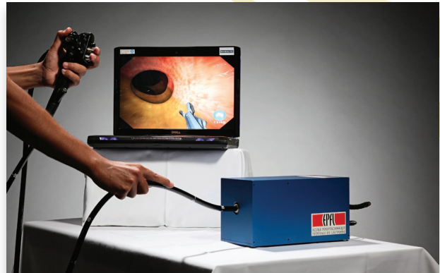
The virtual simulation interacts with a modified clinical endoscope via a high fidelity haptic device.
